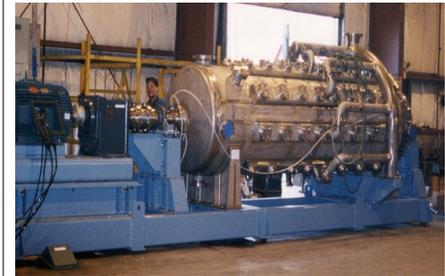
**Quantum Technologies' Liquor Oxidizer reactor is available in 28", 36", 48" diameter and can be engineered and designed to the customer's specifications.**
